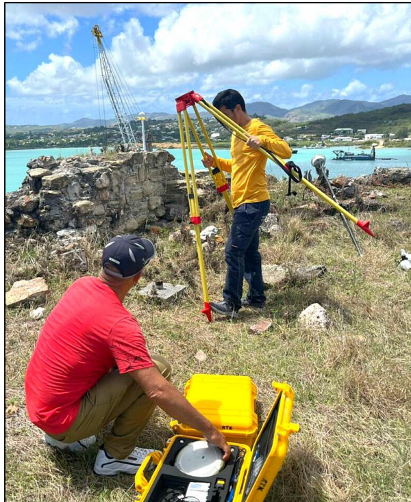
RTK GPS System for Topographic Surveying
