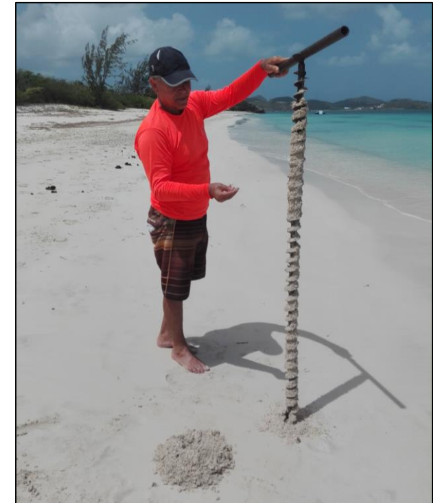
Drilling to check the thickness of the sand layer
