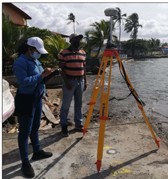
Photo 2. IGNTG specialists during the work to establish the points for the creation of the topographic baseline.
