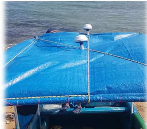
Photo 6. Position of the GPS antennas on the boat
