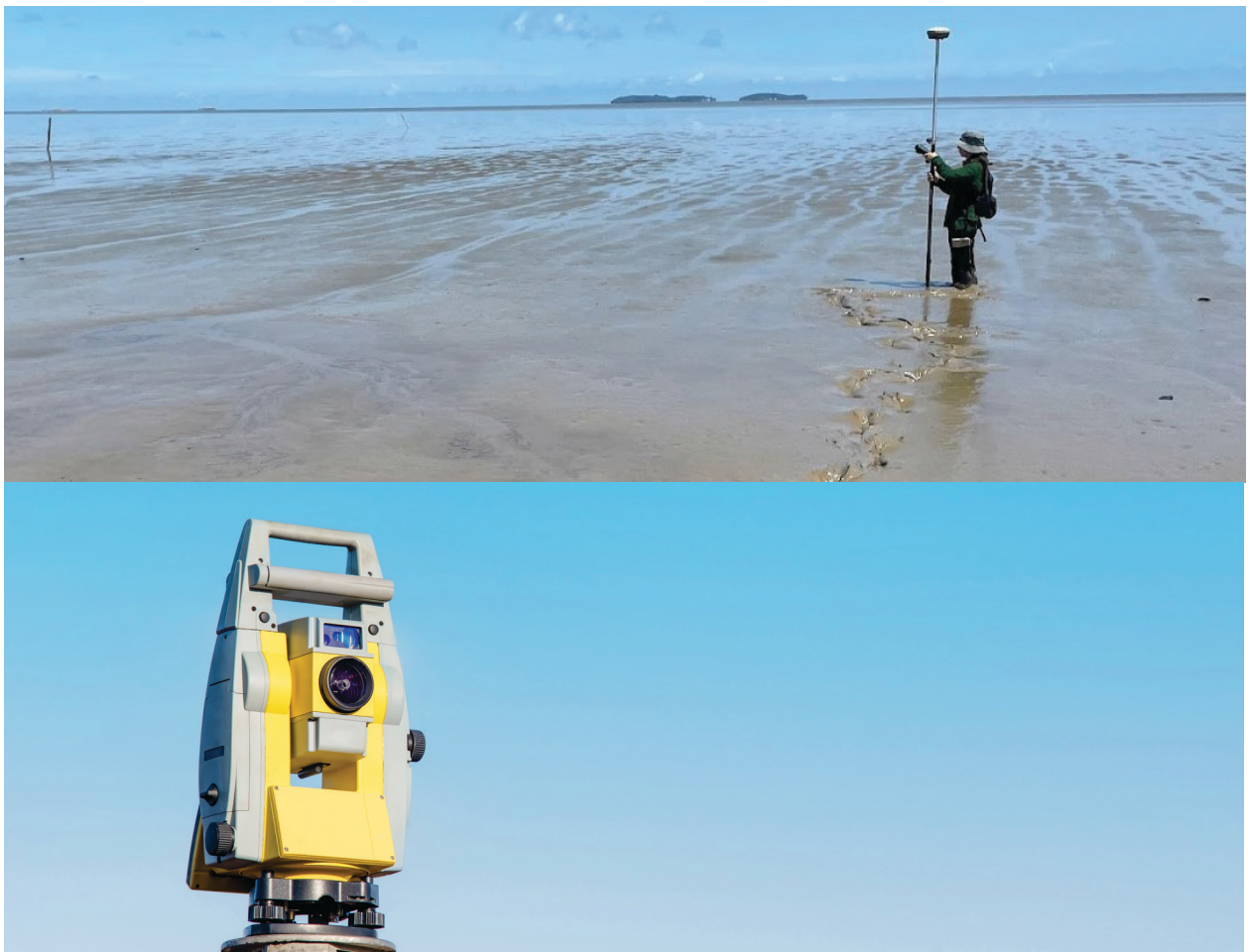
Figure 28 Images of Beach profiling with GNSS systems: fixed and mobile stations
